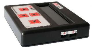
The „classical“ JETIbox generally and the JETIbox mini at the main circuit (cable) requires a pull-up resistor of 10 kOhms between the signal (serial) pin and (+) so that they can be operated directly on the logger. On the JETI-TX-Module they will work without this resistance. When connecting the logger to the front of the JETIbox mini no pull-up is required.
