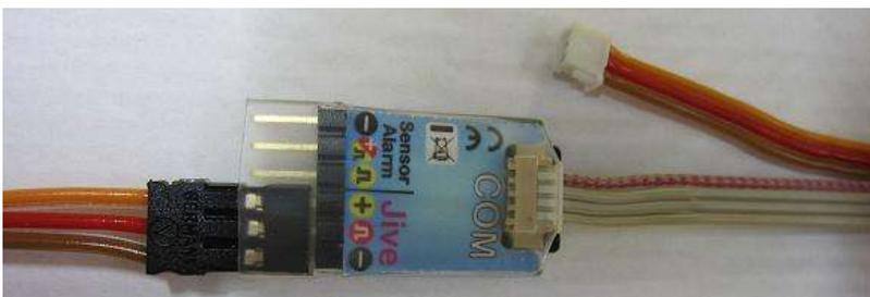
The telemetry cable has three plugs, the smallest one will not be used. This cable is identical to that which **Unilog** uses, here the small plug in addition is connected to **Unilog**, but is left unconnected with *JLog2*.
